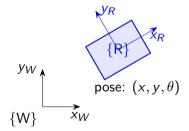
A robot's **pose** in the world is its pos. (x, y) and ori.  $\theta$  w.r.t. the global frame.  $\Rightarrow$  Kinematics allows us to calculate how this pose changes over time.
