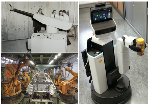
Figure: Two different types of robots. Left: industrial robots, where the upper picture shows the first autonomous and programmable modern robot, the Unimate in 1961, and the lower picture shows the KUKA robot cluster deployed on the automobile production line in 1983. Right: HSR service robot manufactured by Toyota in 2017.
