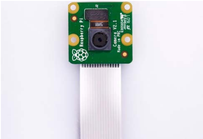
Figure 2 Raspberry Pi Camera v2.1
